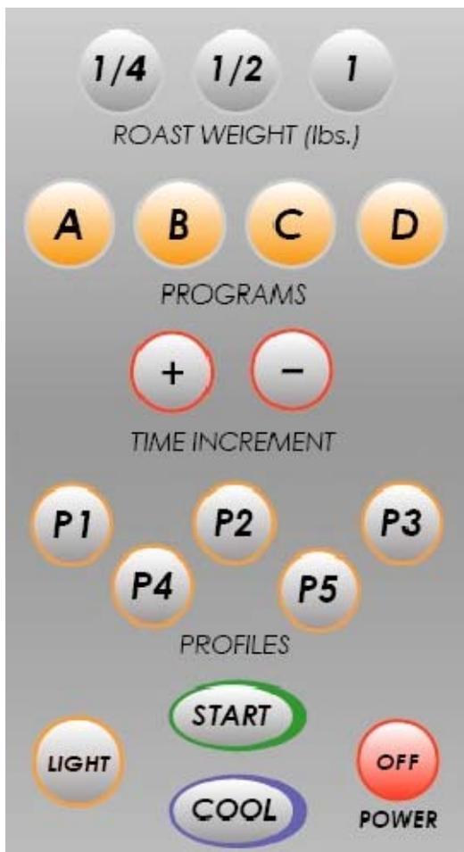
**Roast Weights:** Weight of green coffee beans to be roasted and system on switch. The weight buttons also act as default settings, allowing the user to “reset” the program at anytime before pressing start.
